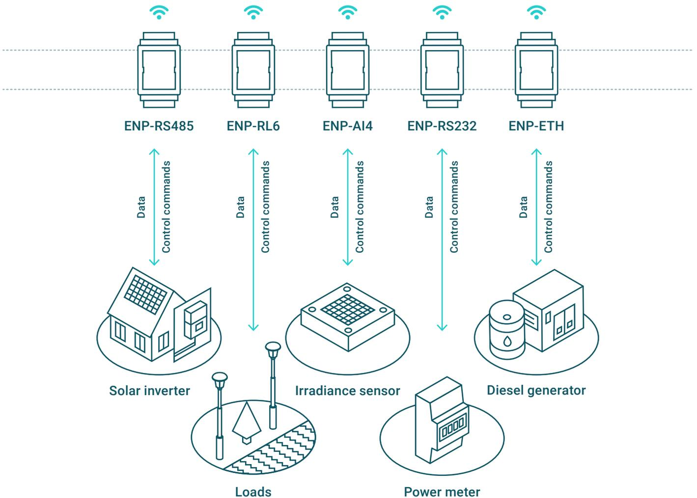
Setup for a renewable energy system with solar inverter connected with an **ENP-RS232 module mounted on 35mm DIN rail according to IEC 60715.**
